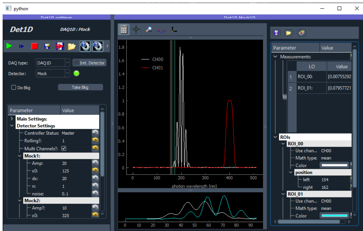
Fig. 7.27: An example of a 1D detector having 2 channels. 0D data are generated as well from the integration of channel CH0 within the regions of interest (ROI_00 and ROI_01).
