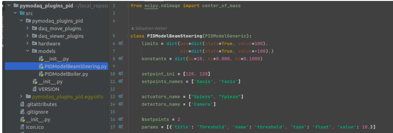
Fig. 7.56: Configuration of a PID model.
