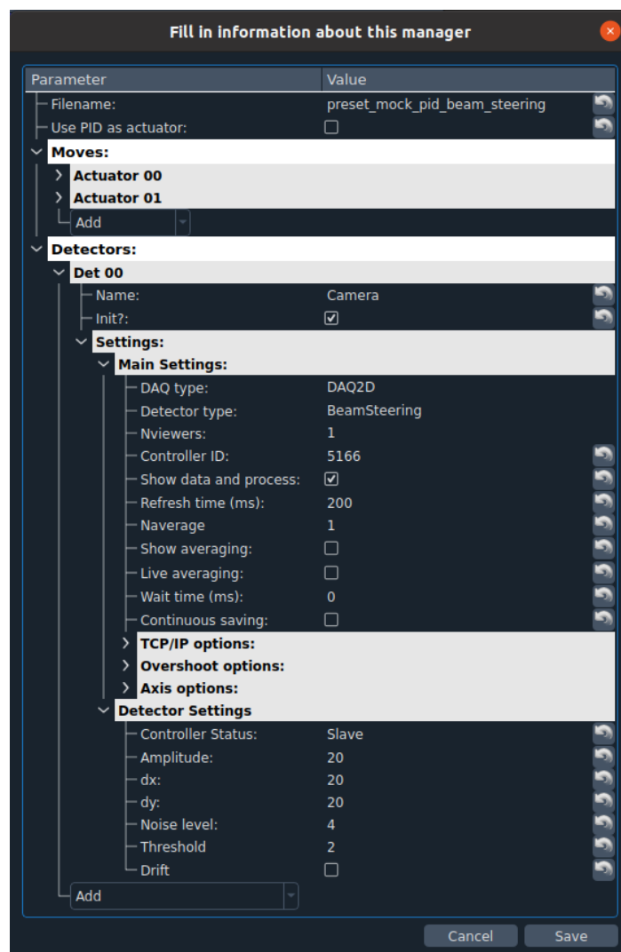
Fig. 7.46: The mock camera configuration.
