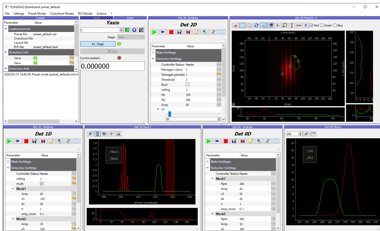
Fig. 7.10: Dashboard user interface containing all declared control modules (actuators/detectors) and some initialization info.
